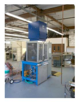
Using high pressure water and garnet to pierce holes in metal products. Uses Trion MP600MHS to collect mist and dust to keep inside of cabinet clean, workers breathing zone free of contaminant and overall work environment cleaner.
